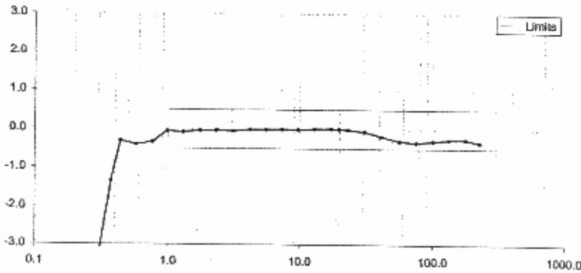
**Isotropy** At frequency of 50 MHz and applied field to 6 V/m the probe is rotated (with 4 degree steps) about the axis of the handle to determine two measurement orientations corresponding to the maximum and minimum sensitivities.
