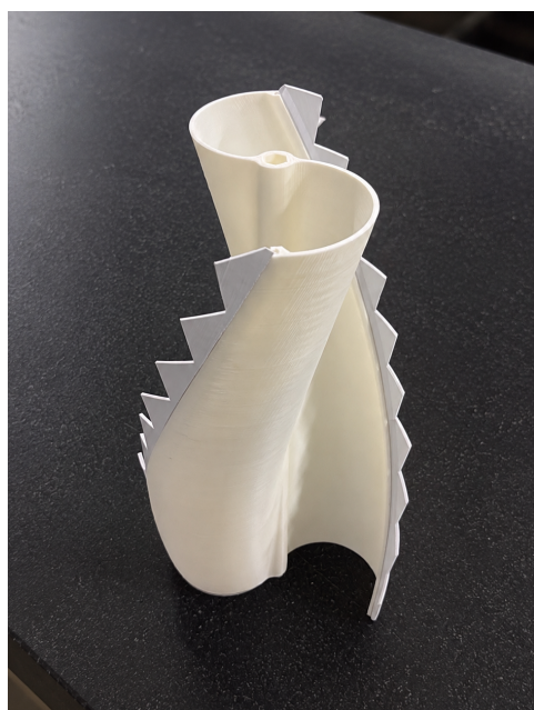
(a) Turbina Chevron impressa
