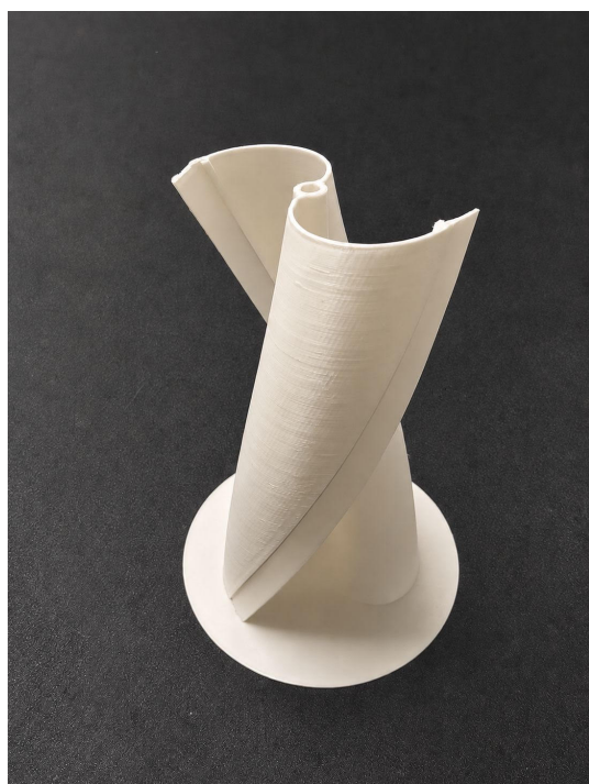
(a) Turbina Bordo Retangular impressa
