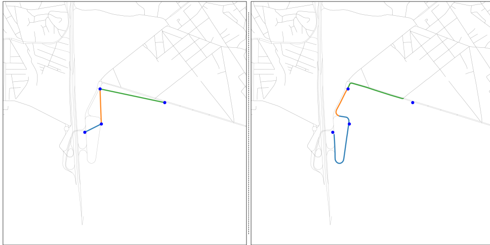
Figure 4.2: Comparison between the trajectory obtained using the Haversine method (left) and the trajectory adjusted by the proposed map matching algorithm (right).
