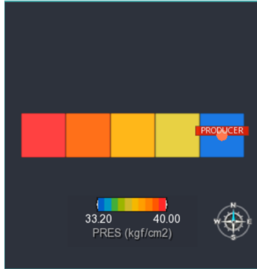
Figure 4.11: Pressure p field at 1000 days simulated. Obtained from GSIM.
