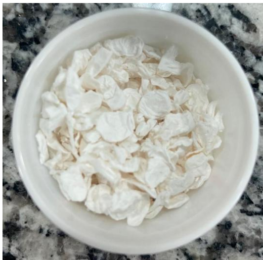
Figure 10: PS/TiO 2 -ACAC composite beads prepared by NIPS methodology.
