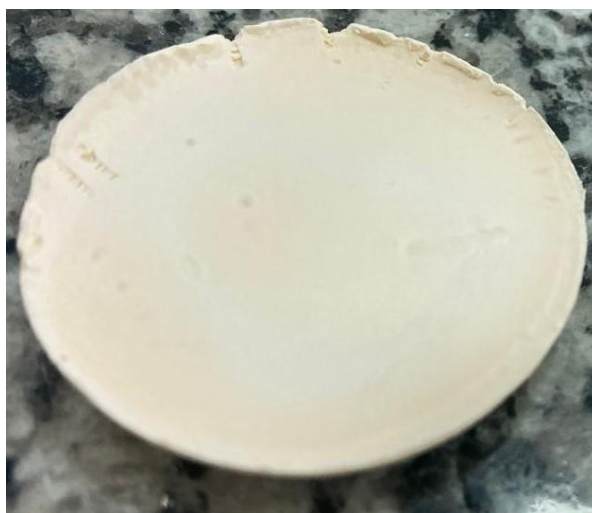
Figure 11: PS/TiO 2 -ACAC composite prepared by TIPS methodology
