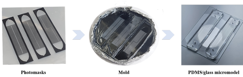
Figure 3.7: Details of the fabrication process of the micromodels.
