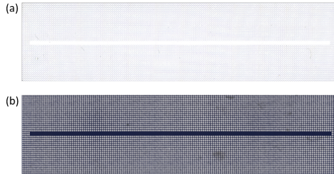
Figure 3.15: Mosaic merge of fractured L2 devices fully filled with: (a) the oleic phase, (b) the aqueous phase.
