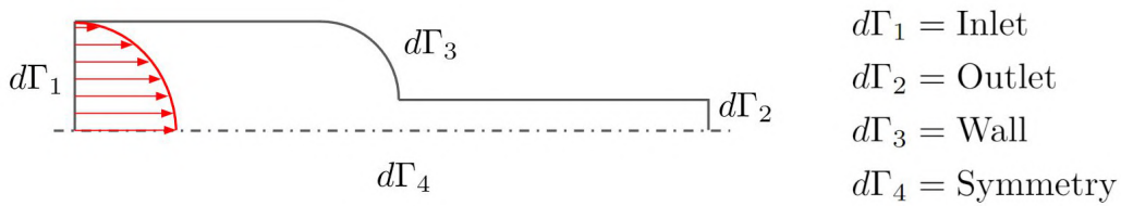
Figure 3.2: Schematic of the flow domain boundary.
