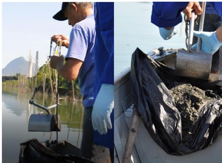
Figure 31 - Sampling collection. A) Van Veen sampler before sampling B) Van Veem sampler after sampling.
