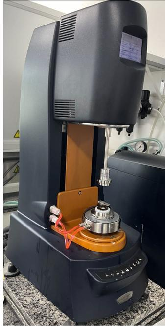
Figura 3.1: Reômetro rotacional *Discovery Hybrid Rotational 3*
