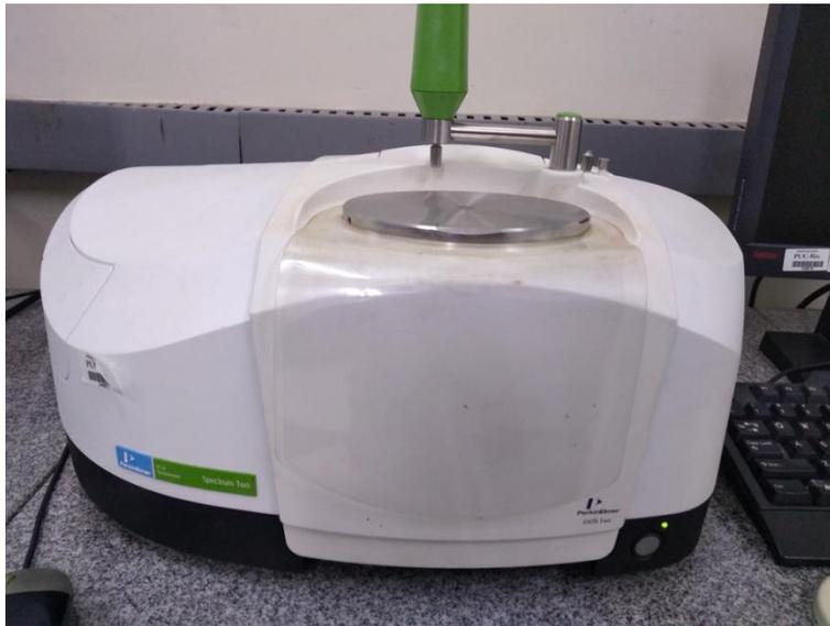
**Figura 3.26.** Espectrômetro FTIR Spectrum Two (*Perkin Elmer*).
