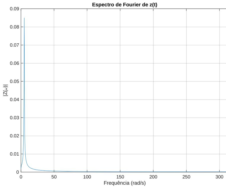
Figura 11: Espectro de Fourier do deslocamento  $z$
