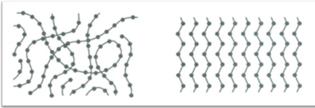
Figure 2-6: Left: Amorphous structures. Right: Crystalline structures (Dowling, 1999).
