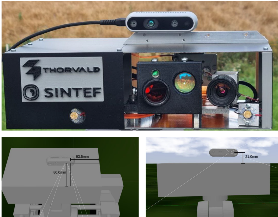
Figure 4.4: Illustration of the Real (up) vs. Simulated (down) Sensors Positioning: 3D Camera and Spectrometer System. The simulated spectrometer system matches the real spectrometer in dimensions, and the coupling of the 3D camera to the sensor also matches the real-world configuration.
