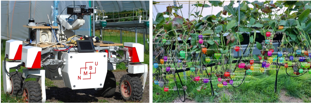
Figure 1.1: The left image shows the mobile manipulator employed in this work, comprising a UGV and a manipulator. The manipulator is equipped with a 3D camera for sensing and detecting strawberries, and a NIR spectrometer for the non-invasive sugar content estimation. The right image shows an example of strawberry detection in a polytunnel environment using the Deep Learning-based vision system.
