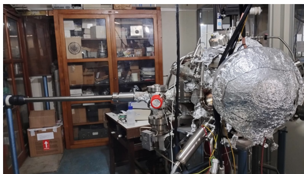
Figure 5.3: X-ray photoelectron spectrometer used to study chemical composition of the samples in the Laboratório de Revestimentos Protetores e Materiais Nanoestruturados at PUC-Rio.
