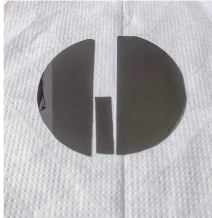
Figure 4.2: Si substrate of 500 \pm 15 micrometers ( \mu\text{m} ) thick cut with a diamond-tipped pen tool in the preferred crystal orientation.
