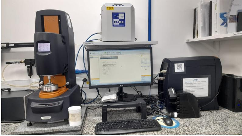
Figure 2.3: Discovery Series Hybrid Rheometer DHR-3.
