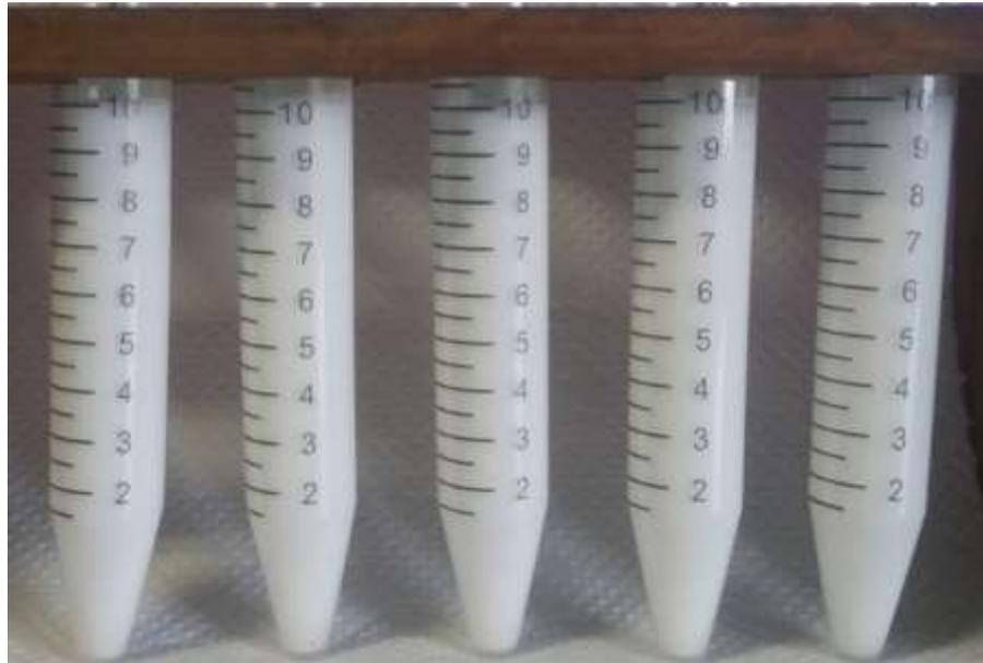
Figure 23. Initial stability of mineral oil in water emulsions using a mixture of surfactants Span®80/Tween®80 at different total surfactant concentration. Pictures taken immediately after preparation.
