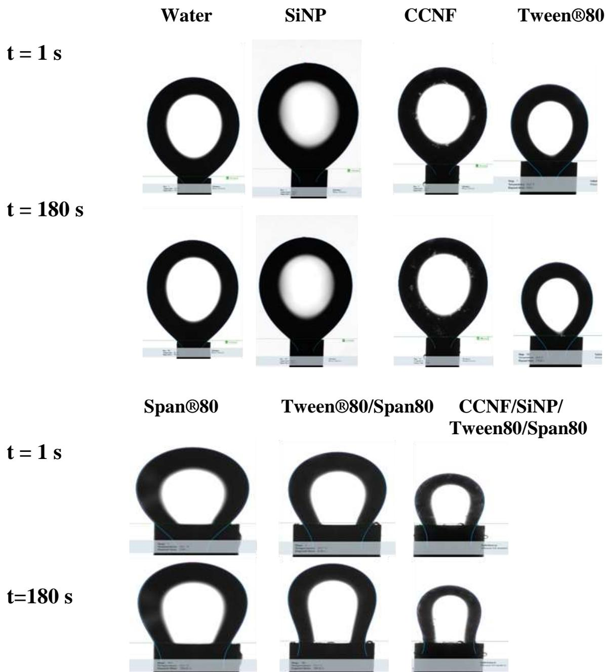
Figure 31. Drop shapes of mineral oil droplet surrounded by aqueous solution/dispersions of emulsion stabilizers.
