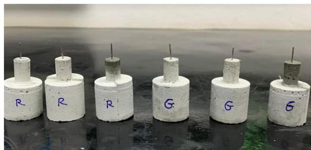
Figure 3.5 – Specimens for the pullout test ("R" for straight and "G" for hooked-end steel fiber).
