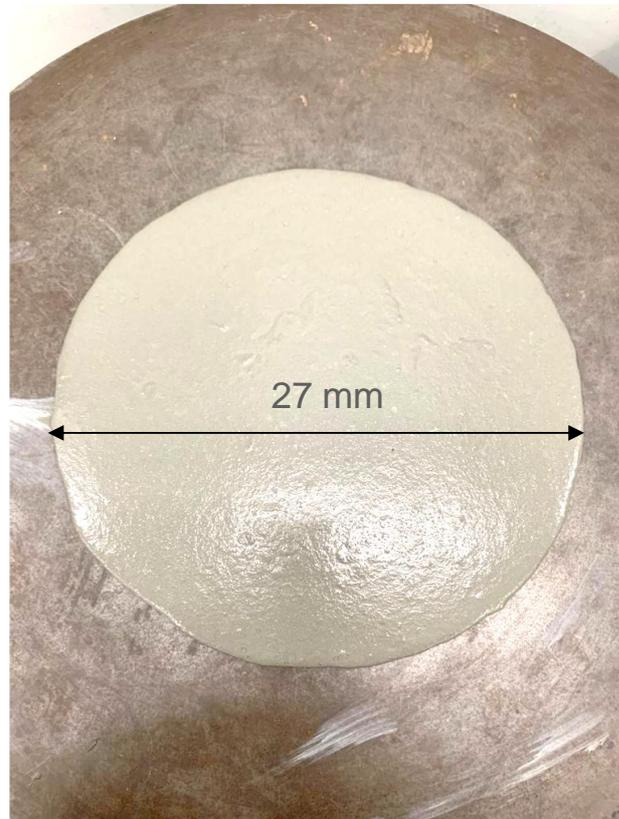
Figure 3.2 – Flow test carried out with Matrix A.
