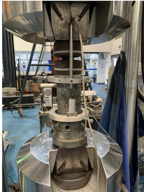
Figure 3.3 – Setup for the uniaxial compression tests in Matrix A.
