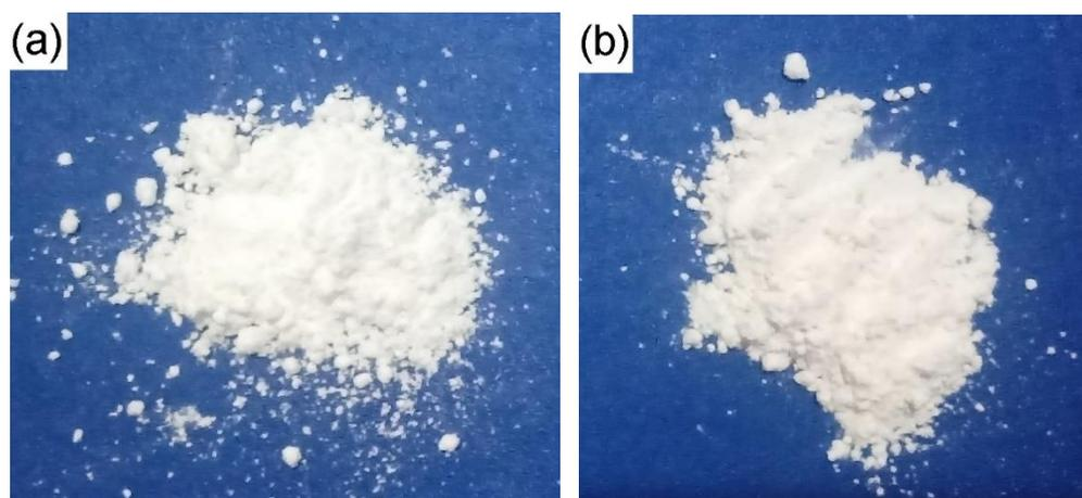
**Figure 5.4** – Visual contrast: (a) nanoclay in its original state as supplied, and (b) nanoclay after heating at 750°C for 2 hours.
