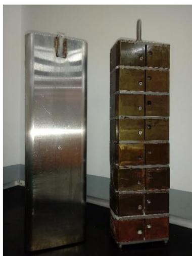
**Figure 4.3** - Set used for autoclave curing: stacked metal molds (on the right) and metal compartment for inserting the molds (on the left).
