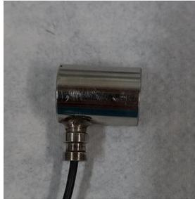
Figure 3.16: Ultrasound transducer of the experiment.
