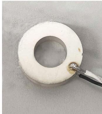
Figure 5.19: Cylindrical transducer for the experimental test.
