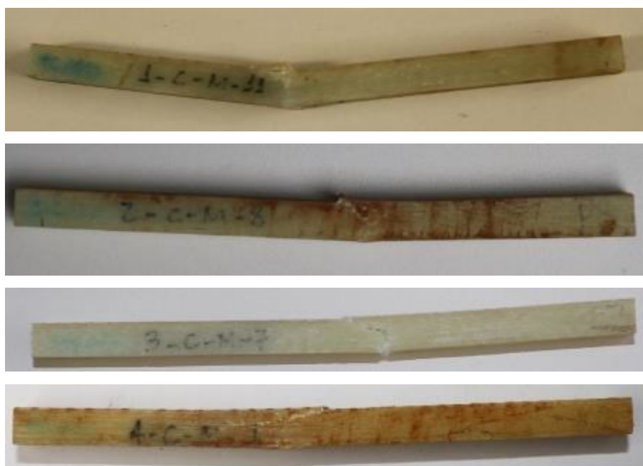
B. 3. Failure modes for the aged bending specimens (R1 – R7) at 55°C.
