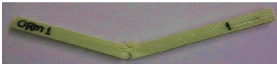
B. 1. Failure mode for the unaged bending specimens.
