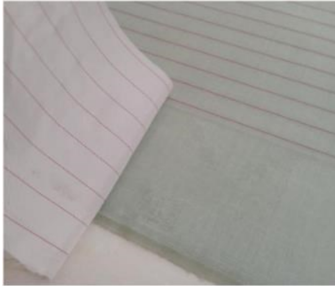
A. 4. Application of a peel-ply fabric layer [155].
