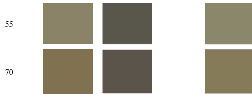
Figure 137. Evolution of color for the three materials with temperature and time.
