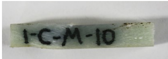
B. 7. Failure modes for the aged ILSS specimens (R1 – R7) at 55°C.
