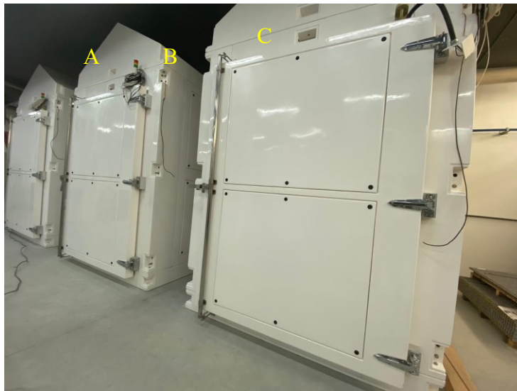
Figure 60. Salt-spray chambers and identification adopted.
