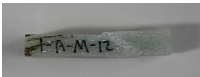
B. 5. Failure mode for the unaged ILSS specimens.
