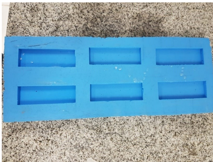
Figure 59. Silicon mold used to fabricate the epoxy specimens for absorption tests.
