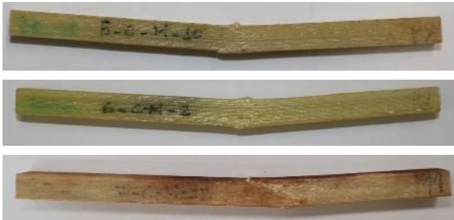
B. 4. Failure modes for the aged bending specimens (R1 – R7) at 70°C.
