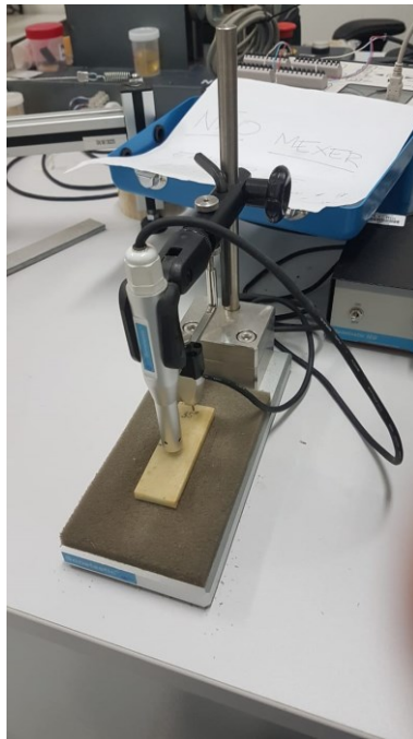
Figure 66. Sonelastic ® equipment used for IET test.
