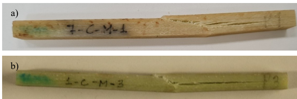
Figure 118. Delamination failure modes observed in few specimens. (a) 10170-hours aged specimen (R7) at 70°C and (b) 570-hours aged specimen (R1) at 70°C.
