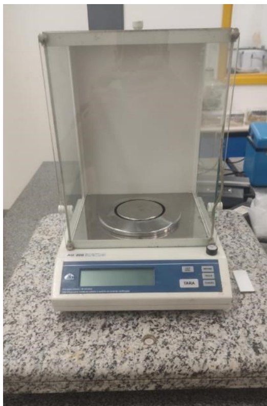
Figure 63. Weighing balance used in the gravimetric tests.
