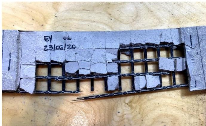
**Figure 4.15** – TRC with the EP fabric after the direct tensile test.
