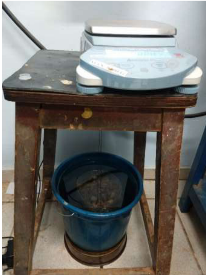
Figure 3-9. Saturated aggregate submerged in water and hydrostatic scale.
