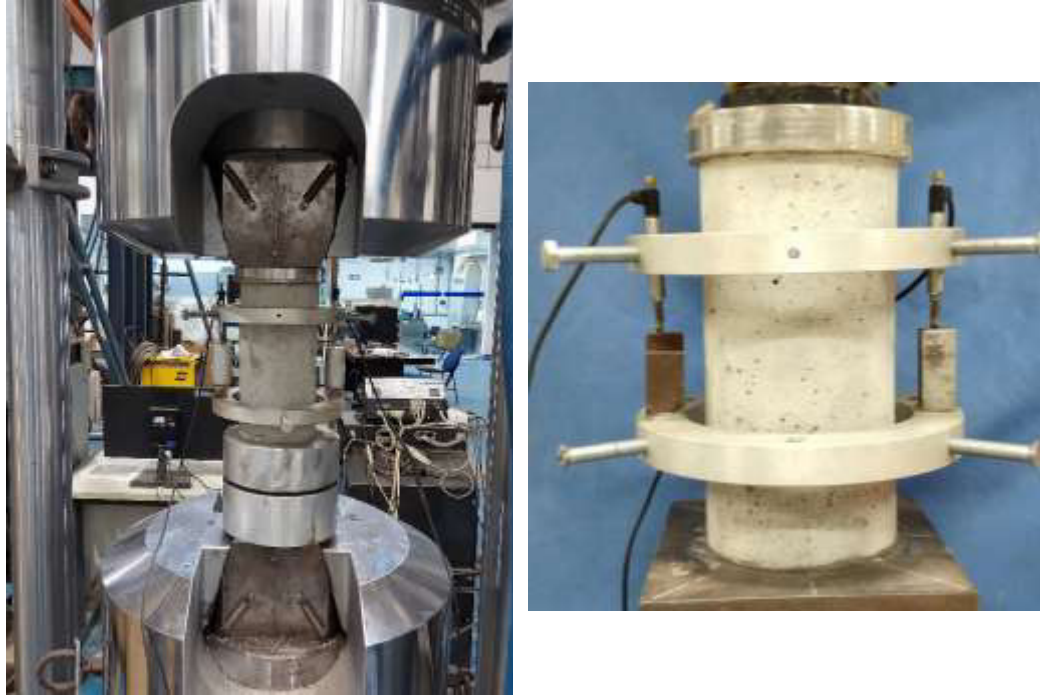
Figure 4-14. Compressive strength test performed on a 500 kN servo-hydraulic MTS actuator.
