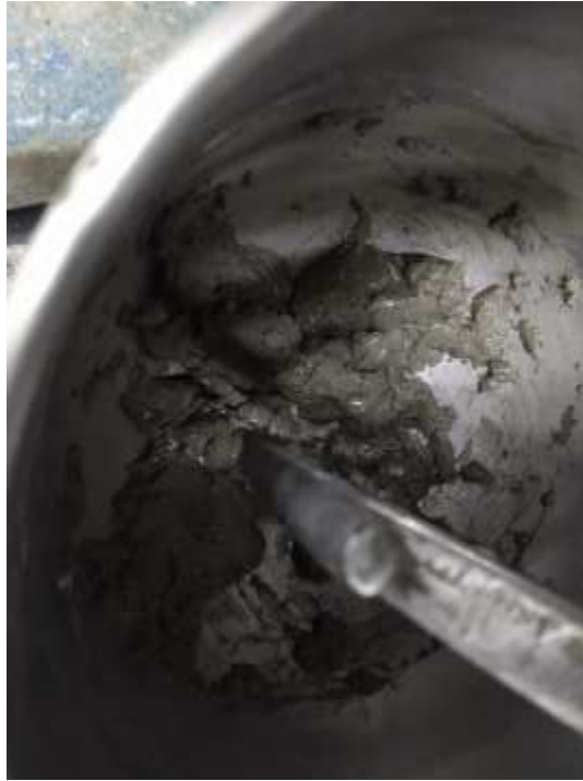
Figure 4-7. Capillary state, characterized by a homogeneous paste and no moisture on the mixer's wall.
