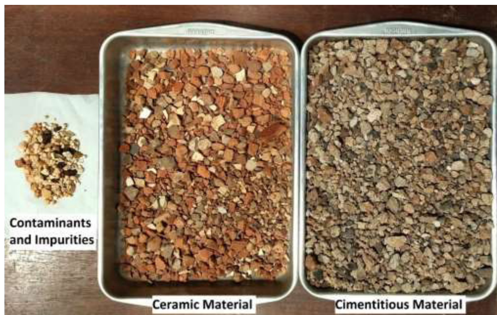
Figure 3-4. Sample of recycled aggregate separated into three groups: contaminants and impurities, ceramic material, and cementitious material.
