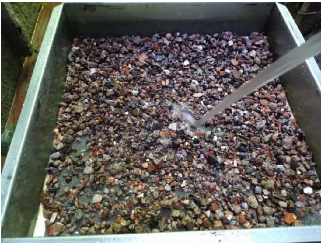
Figure 3-2. Recycled aggregate cleaning process with running water.
