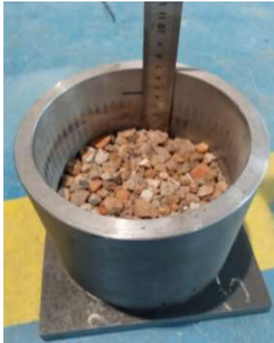
Figure 3-11. Measurement of the distance between the surface of the aggregate and the top of the steel cylinder container.
