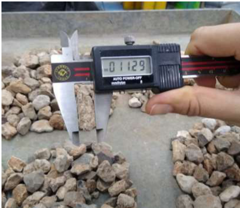
Figure 3-6. Digital caliper used to measure the length and thickness of coarse aggregate grains.
