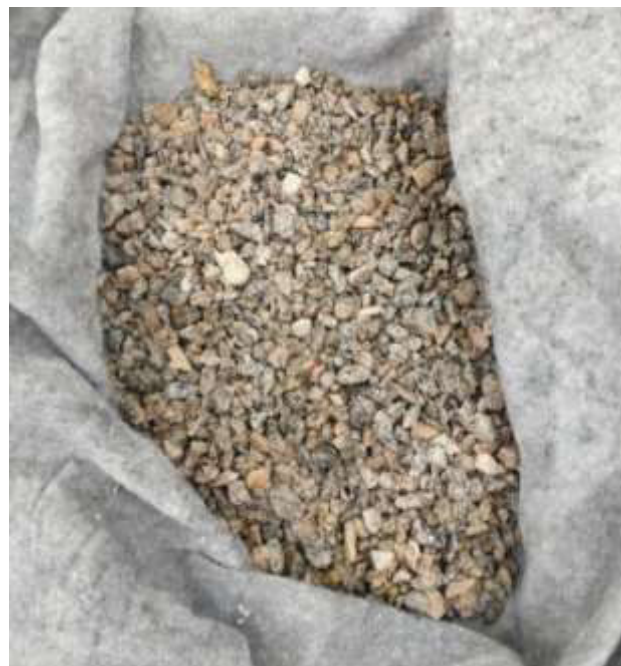
Figure 3-8. Aggregates being rolled in a large absorbent tissue.
