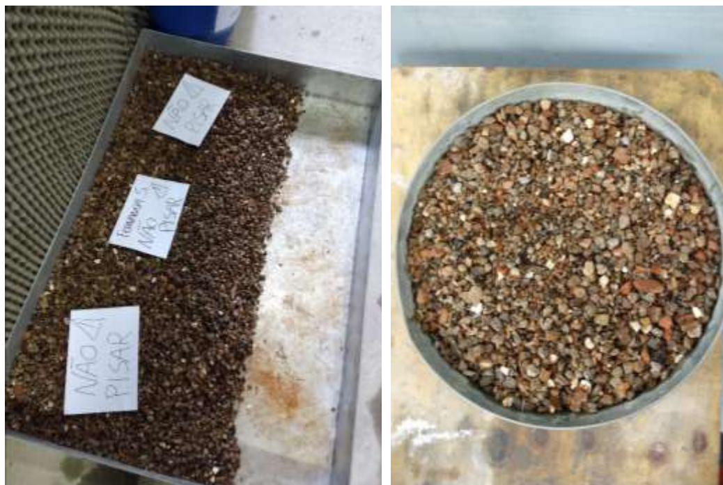
Figure 3-3. Recycled aggregate air-drying process.
