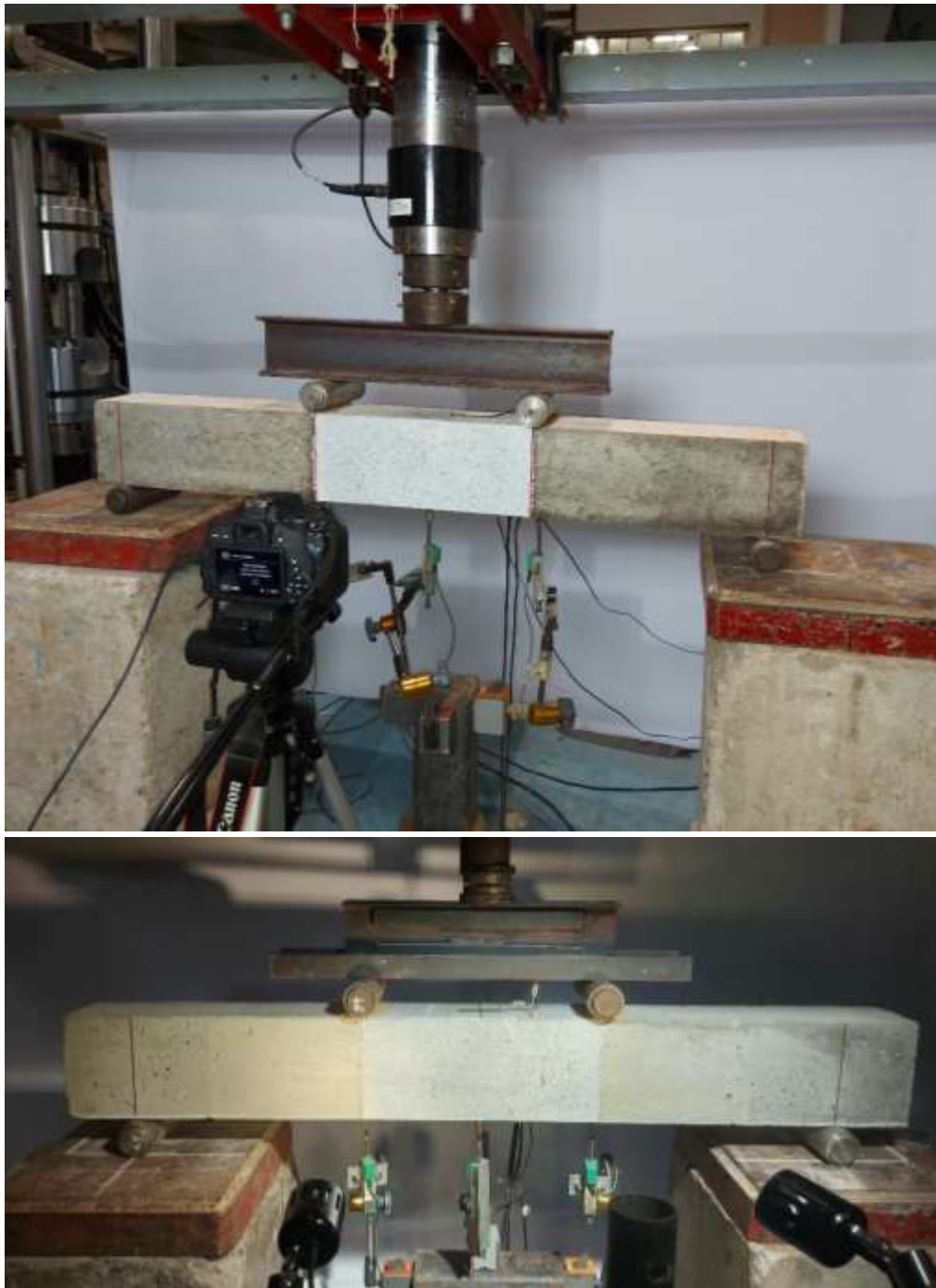
Figure 5-5. Beam positioned for the four-point bending test.
