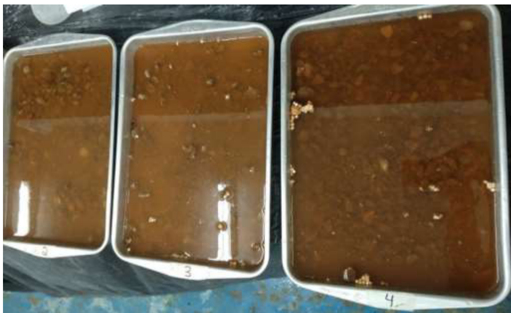
Figure 3-5. Mixed recycled aggregate samples during pulverulent content test.
