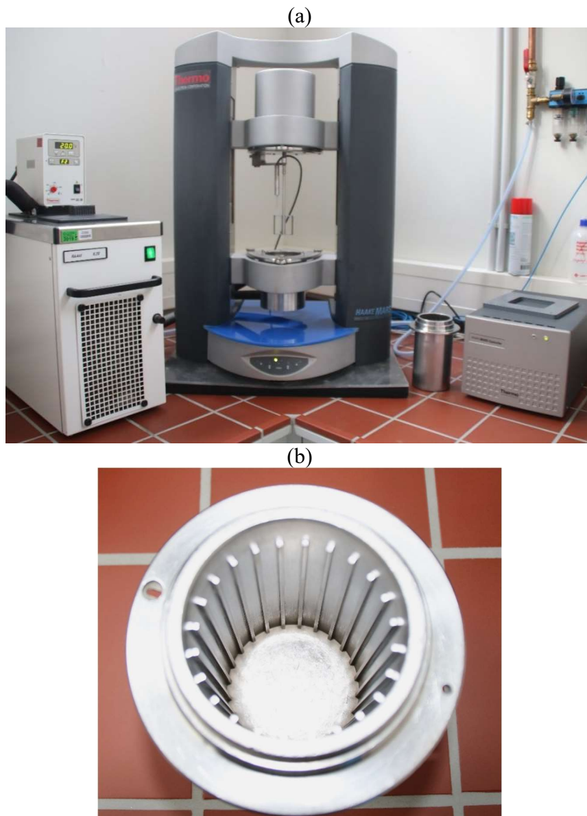
Figure 6-1 (a) The rheometer used coupled with a temperature control module. (b) The cell unit.
