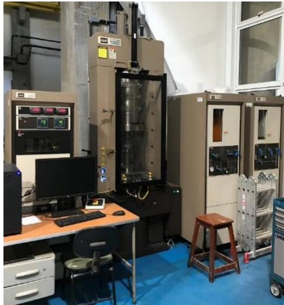
Figure 4-4 – MTS triaxial system used for the multi-stage triaxial compressive tests.
