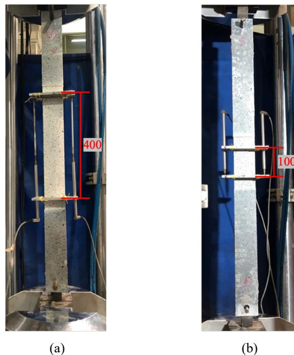
**Figure 4.5 - Tensile test with steel tabs glued with different gauge lengths.**
