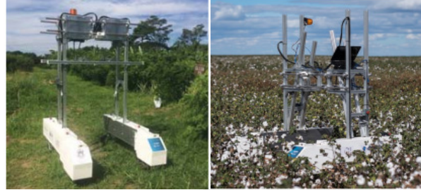
Figure 1.2: (a) Soybot, a mobile robot designed for inspection of soy and cotton crops ; (b) Soybot monitoring a cotton crop .
