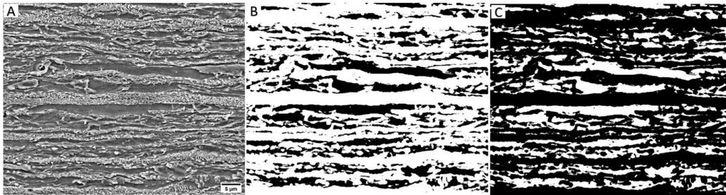
Figure 5.3 WEKA segmentation of the cold rolled steel. A – Original 2000X image. B – Pearlite. C – Ferrite.
