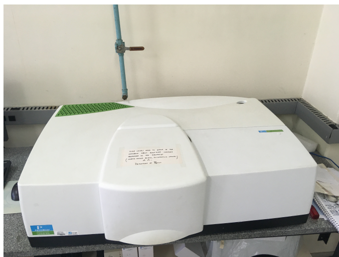
Figure 3.5: Spectrophotometer from Perkin–Elmer (USA, model Lambda 950) in the Optical Spectroscopy Multiuser Laboratory of the Department of Physics of PUC-Rio.
