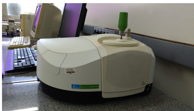
Figure 3.6: Spectrophotometer Spectra-Two (Perkin Elmer, U.S.A.) in the Optical Spectroscopy Multiuser Laboratory of the Department of Physics of PUC-Rio.
