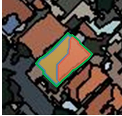
Figure 6: Two possible merging regions, C_1 (blue) and C_2 (red), and the final result C_1 \cup C_2 (green).
