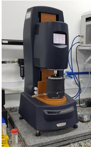
Figure 3.8: Parallel plate rheometer used for rheology tests.
