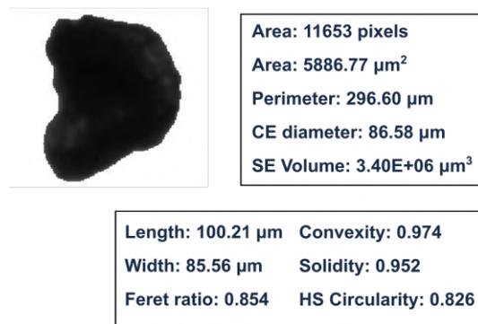
Figure 4.4: Example: soapstone particle and the corresponding values for the size and shape parameters measured.
