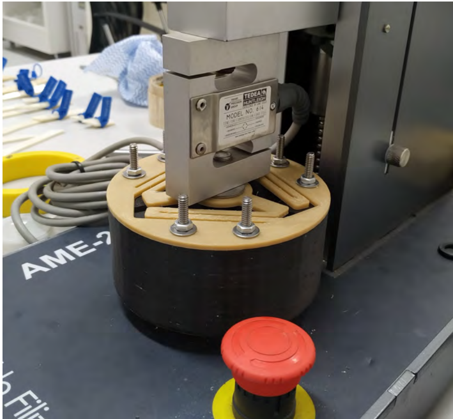
Figure 3.11: Mechanical testing setup of an ortho-planar spring.
