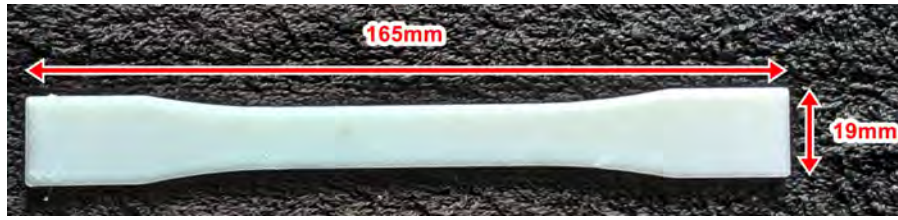
Figure 3.2: 3D printed tensile type I specimen.
