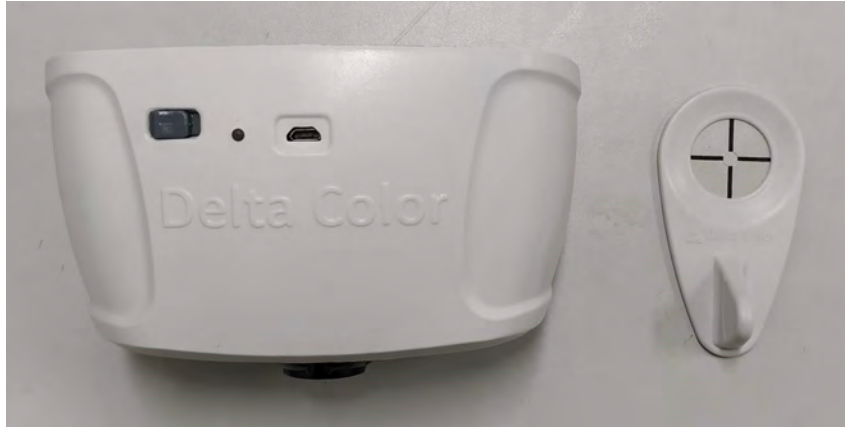
Figure 3.13: Colorimetry equipment Delta Vista from the company Delta Color used in the tests.
