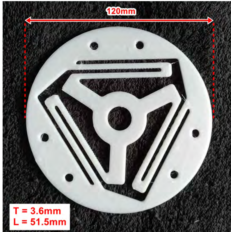
Figure 3.4: Printed ortho-planar spring mechanism with 6 auxiliary holes.
