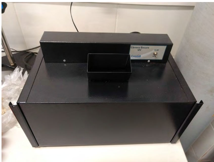
Figure 3.8: UV dark chamber used in the ultraviolet radiation aging.
