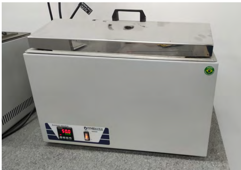
Figure 3.9: Water bath equipment used in the water and oil immersion agings.
