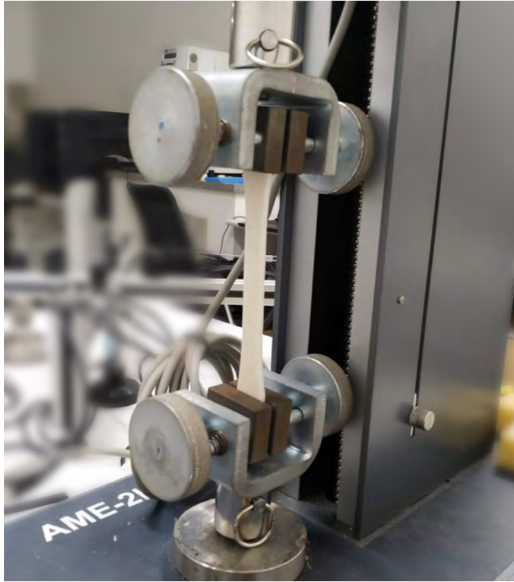
Figure 3.12: Tensile sample placed in the AME-2kN universal testing machine for the tensile test.
