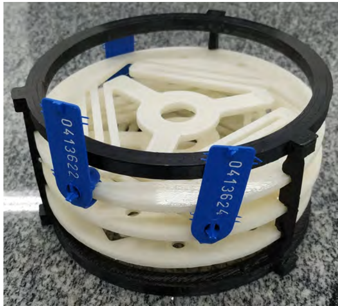
Figure 3.5: Setup for the water and oil immersion agings of the ortho-planar spring with auxiliary printed parts.
