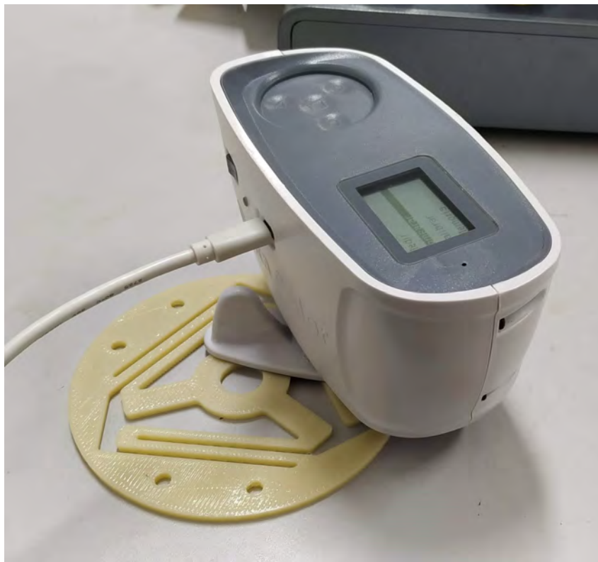
Figure 3.14: Colorimetric test of an ortho-planar spring.
