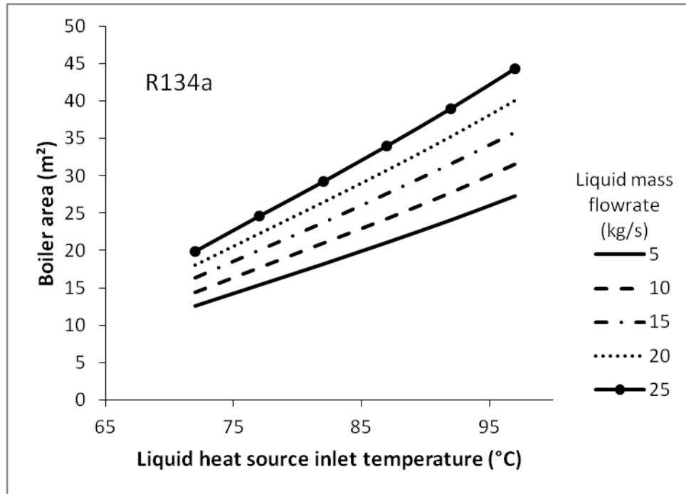
Figure 20. PHE boiler area using R134a at a high pressure of 15.52 bar.
