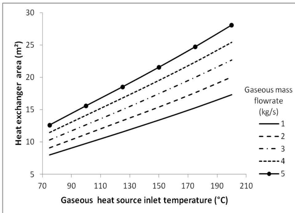
**Figure 24. Tube-fin heat exchanger using R245fa at a high pressure of 16 bar.**
