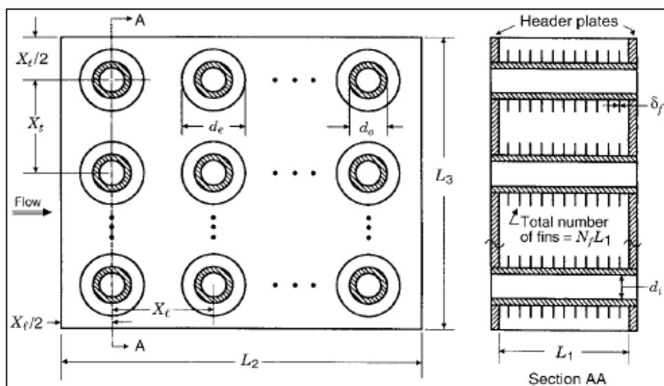
**Figure 16. Circular-finned tubular exchanger, from Shah [26].**
