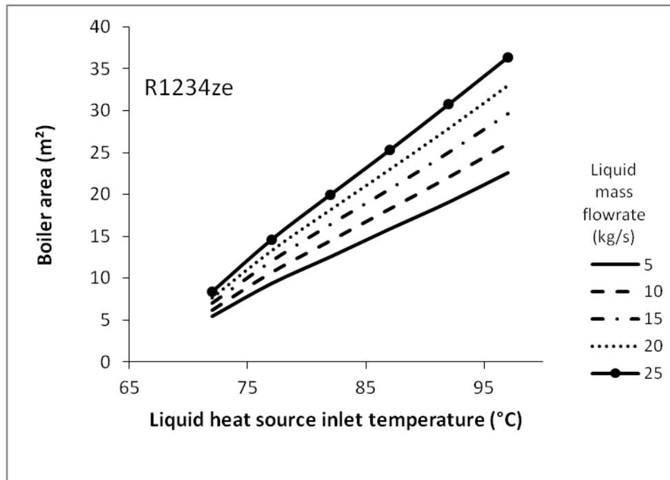
**Figure 22. PHE boiler area using R1234ze at a high pressure of 15.34 bar.**
