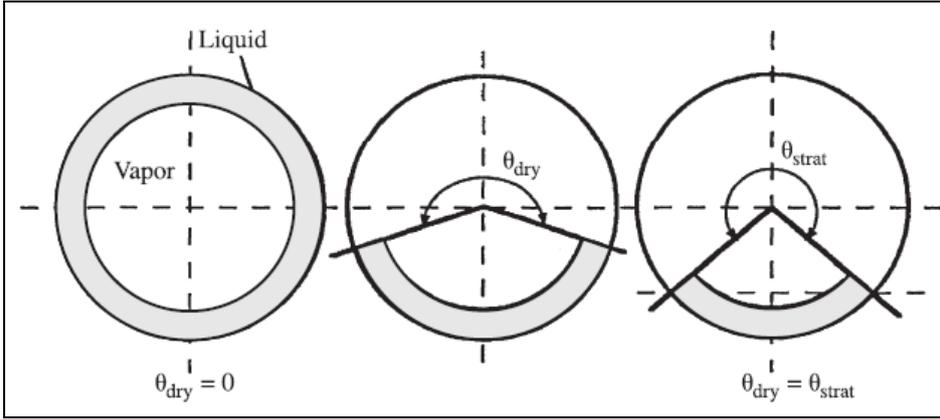
**Figure 19. Transition from annular flow to stratified flow, Kattan et al. [45].**
