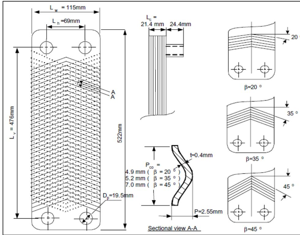
Figure 15. Schematic diagram of a brazed plate heat exchanger [43].
