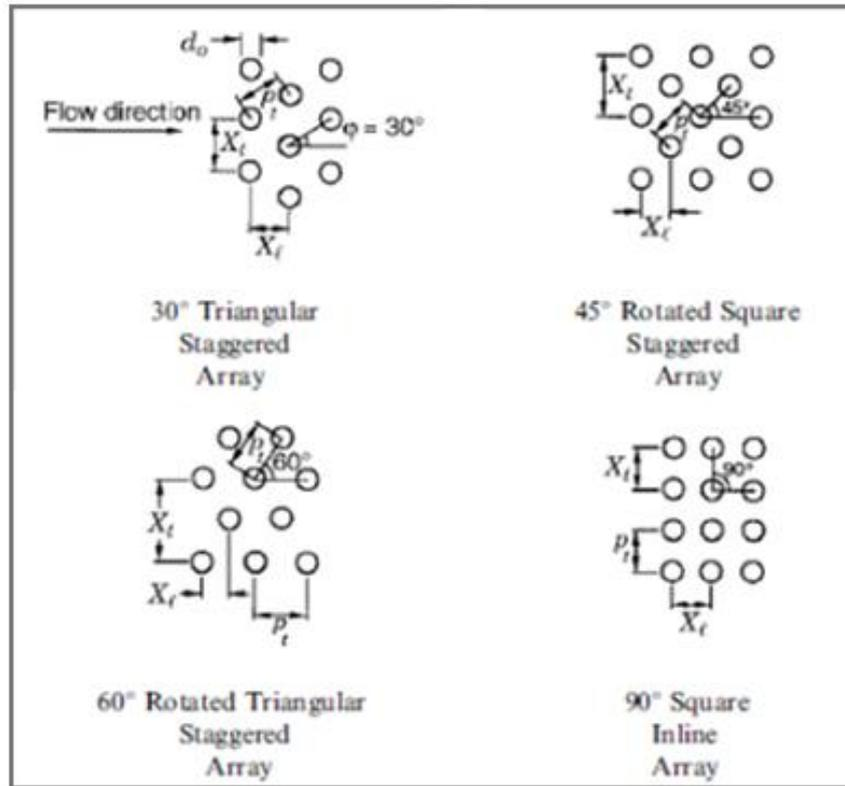
**Figure 17. Various geometrical tube layout arrangements, from Shah [26].**
