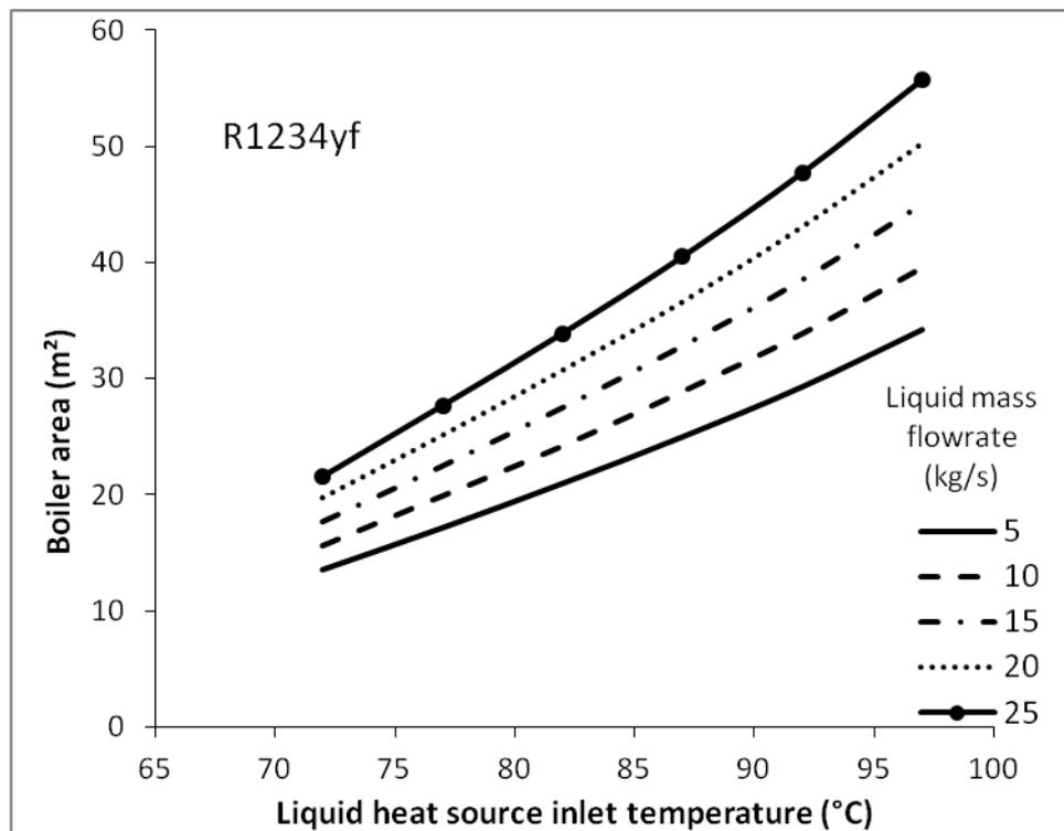
Figure 21. PHE boiler area using R1234yf at a high pressure of 15.56 bar.
