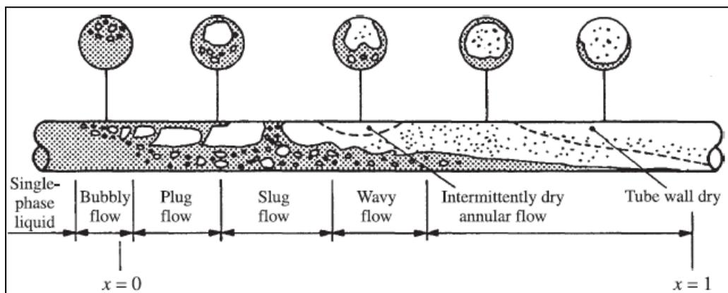
**Figure 18. Two-phase flow patterns during evaporation in a horizontal tube, Collier and Thome [45].**
