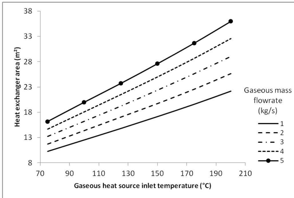
**Figure 25. Tube-fin heat exchanger using R123 at a high pressure of 16.3 bar.**
