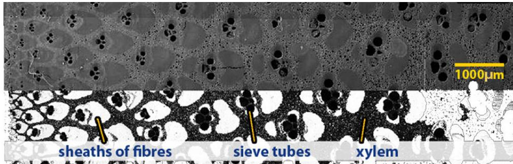
Figure 2.1- Transverse section of *Dendrocalamus giganteus* (DG) bamboo showing a decreasing distribution density of vascular bundles from the outer layer to inner layer of the culm wall
