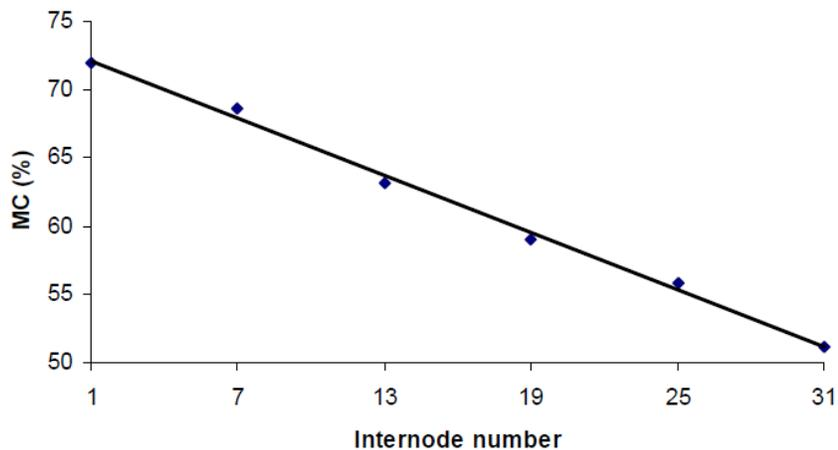
Figure 2.2- Moisture content of three years old bamboo of different internodes [43]
