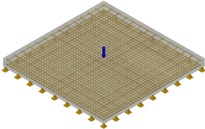
Figure 2.6 - Full scale two-way concrete slab reinforced with bamboo strips scheme
