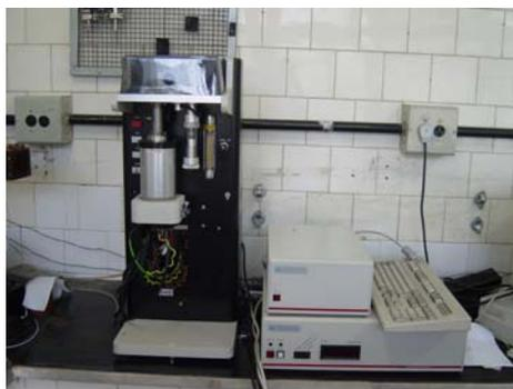
Figura 5.17 – STA 1500 da Polymer Laboratories.
