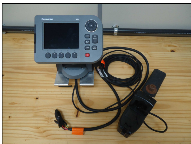
Figura 3.6 – Monitor do GPS e Sonar modelo A50D 5" Chartplotter/ Fishfinder .
