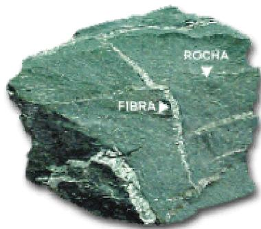
Figura 2-3 Mineral asbesto bruto (INCA, 2002).
