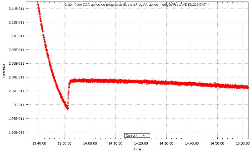
Figure 25: Typical freezing plateau of the silver fixed point cell
