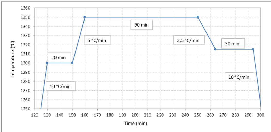
Figure 18: Heating and cooling program for Thermal Technologies furnace
