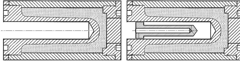
Figure 24: Original (left) and modified (right) silver blackbody cavity
