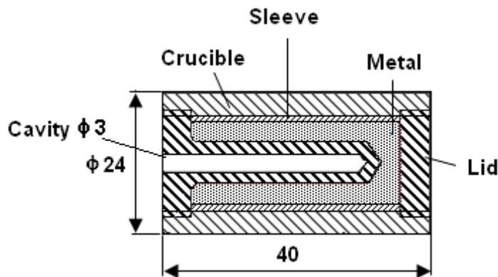
Figure 10: Blackbody cell design used in this study – dimensions in millimeters
