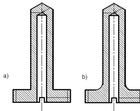
Figure 16: Blackbody cavities – (a) Old model (b) New model
