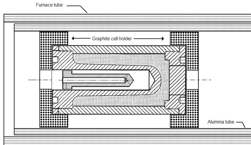
Figure 23: Assembly of the silver cell inside the furnace
