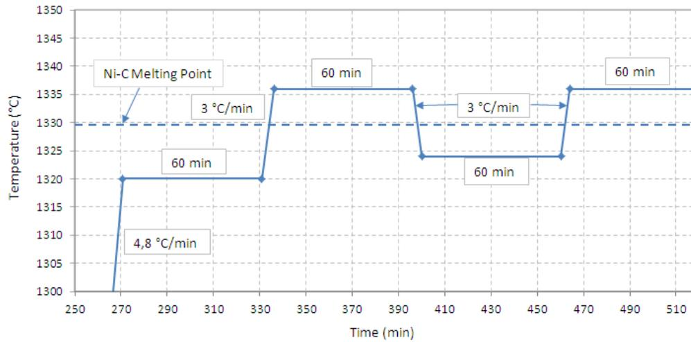
Figure 21: Heating/cooling program of the Carbolite TZF18 furnace
