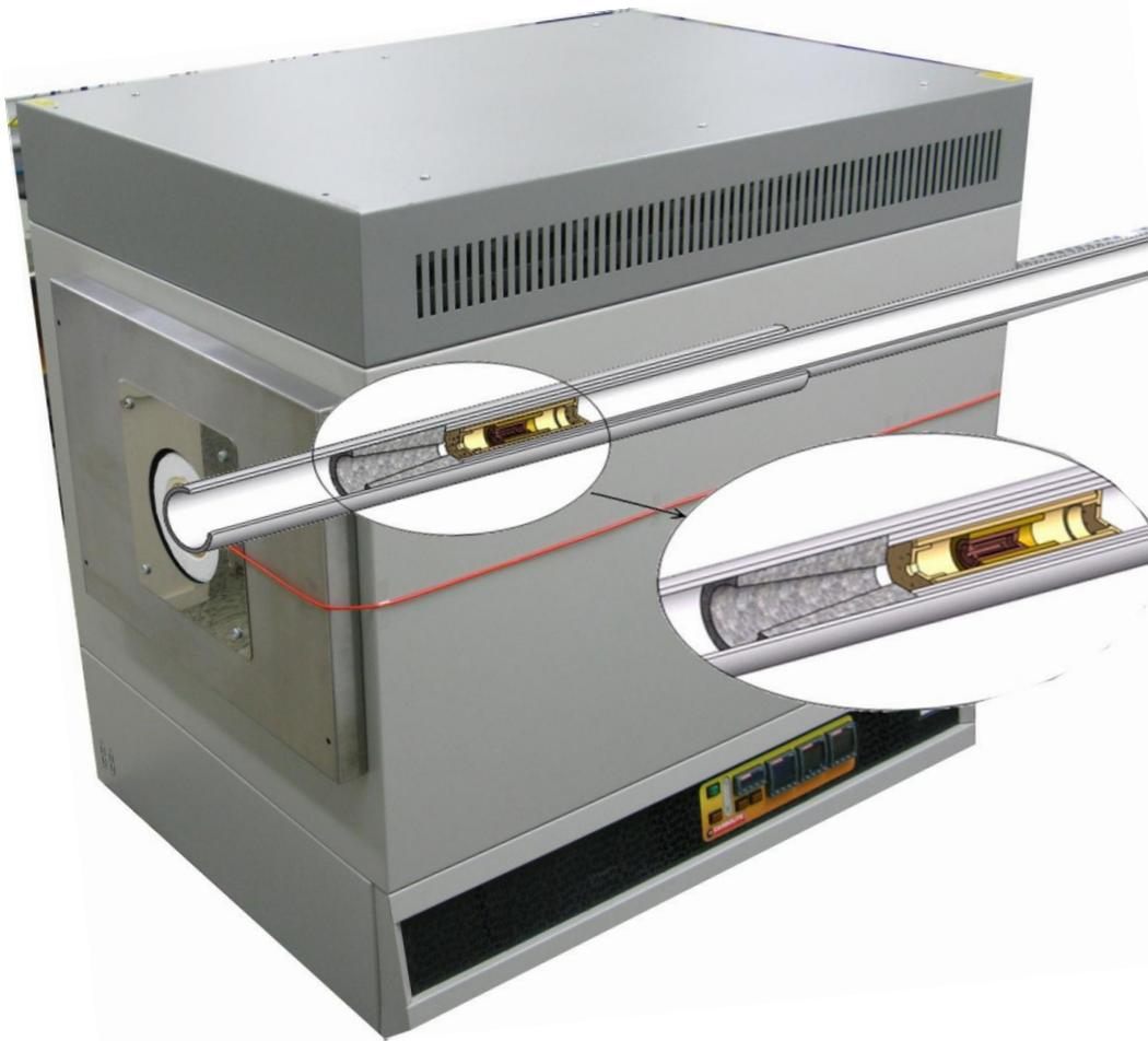
Figure 22: Assembly of the eutectic cell inside Carbolite TZF 18 furnace
