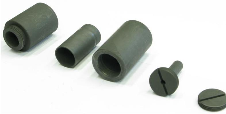
Figure 11: Parts of the eutectic cell
