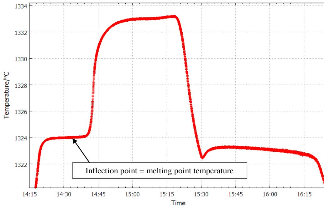
Figure 17: Typical realization curve of the Co-C eutectic in the carbolite 3-zone furnace
