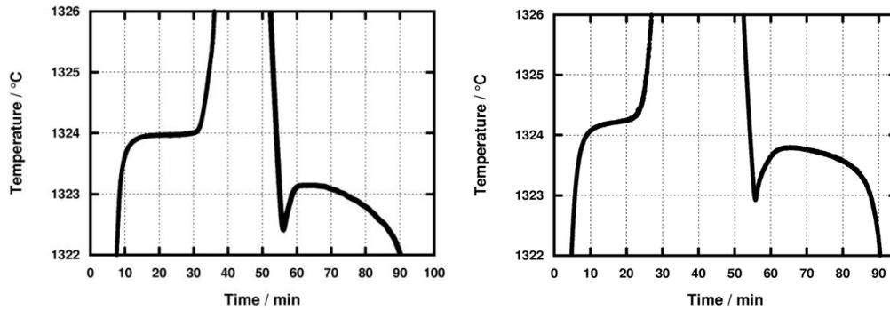
Figure 15: Realization of Co-C (left) and Co-C-Cu (right) eutectics
