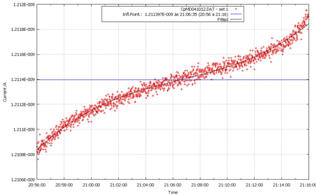
Figure 14 - Example of the determination of the point of inflection of the melting curve of the Ni-C eutectic.
