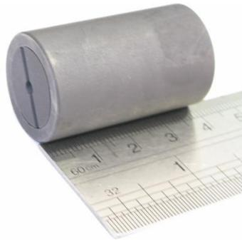
Figure 12: Typical eutectic cell
