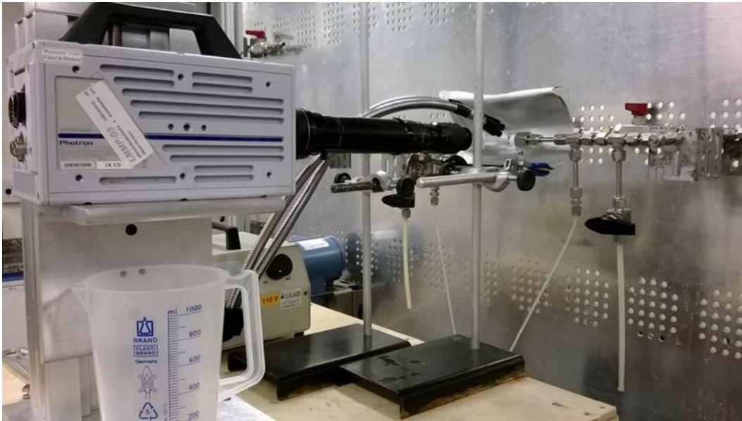
Figure 3. 10 Experimental set-up for the visualization of breakup mechanisms in the flow through an orifice. Single droplet case.
