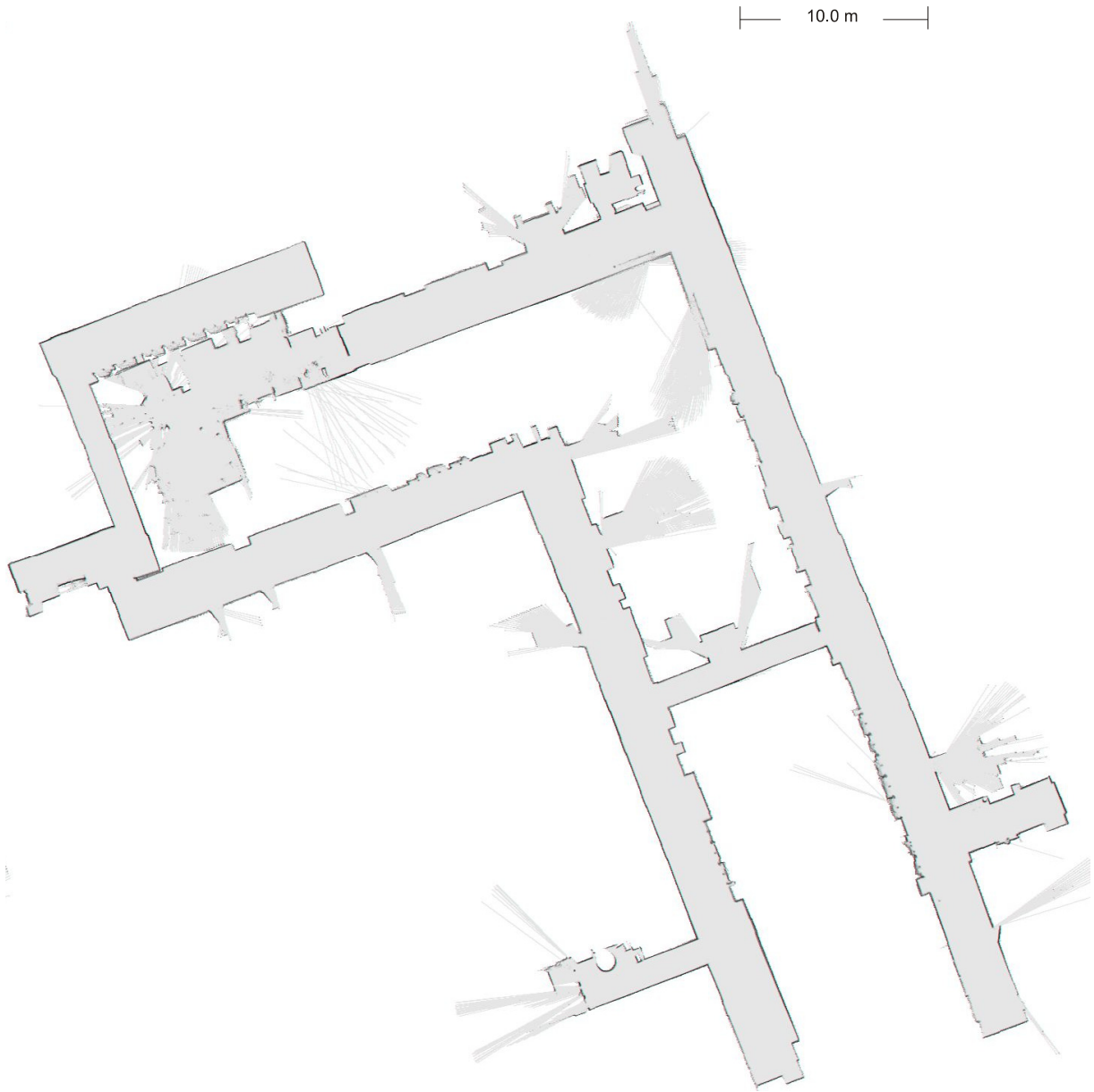
Figure 5.32: 2D grid map of “Diiga” experiment, acquired with DP-SLAM using the proposed motion model.
