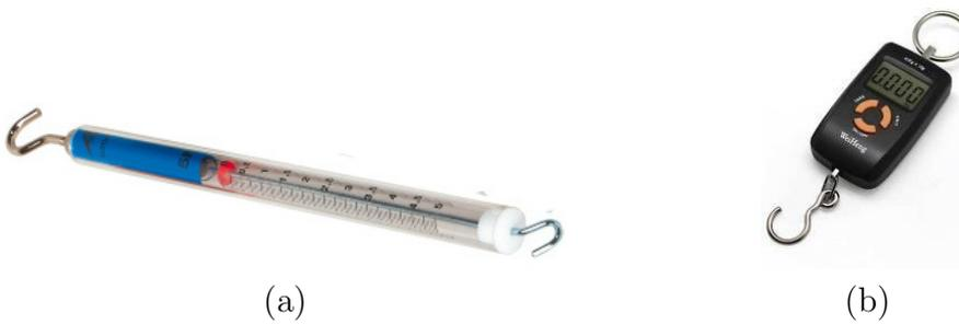
Figure 4.9: Used dynamometers of (a) 3B U20034 of 5 N (0.05 N of precision) and (b) Weiheng of 40 kg (0.01 kg of precision).
