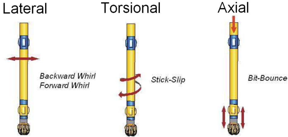
Figure 1.4: Drillstring vibration [29].
