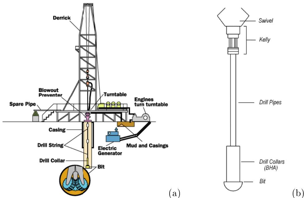
Figure 1.2: Sketches: a) drilling rig (website www.howstuffworks.com); b) oil well drillstring.
