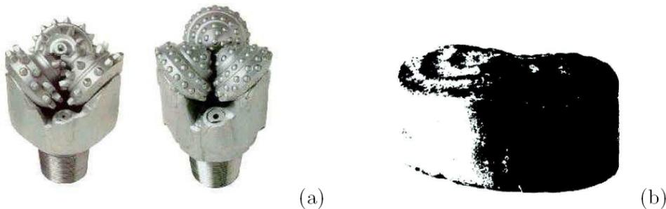
Figure 1.5: a) Roller cone bit (website [geocities.yahoo.com.br/perfuracao](http://geocities.yahoo.com.br/perfuracao)); b) trilobe formation on hard rocks caused by roller cone bits drilling [25].
