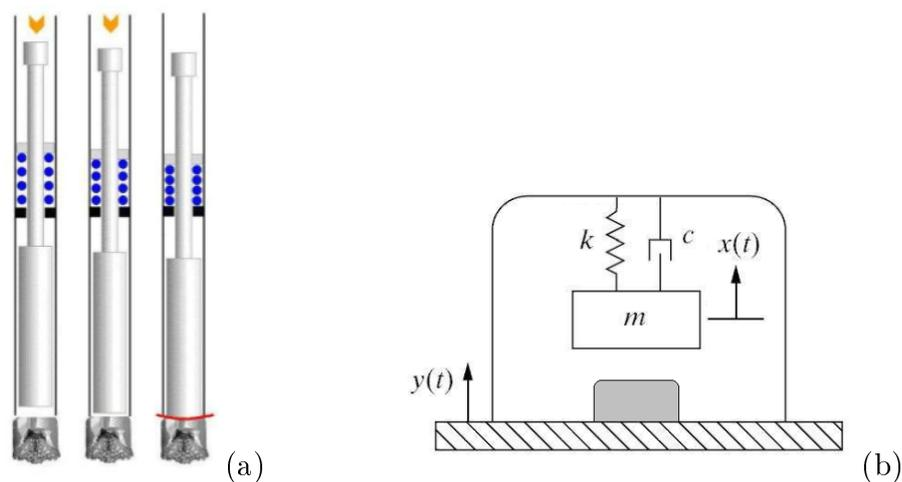
Figure 1.6: a) Resonance Hammer Drilling (RHD) technique [29].; b) Vibro-impact system.
