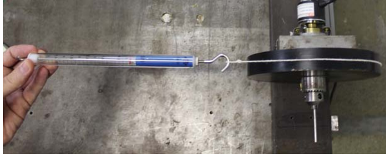
Figure 4.8: Experimental torque measurement
