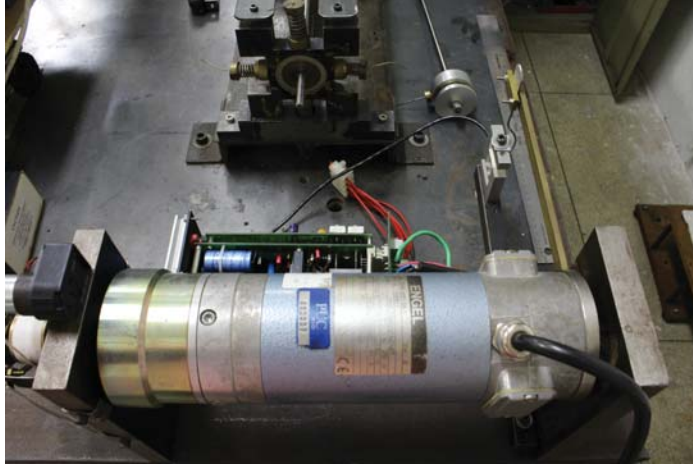
Figure 4.3: Top drive DC motor
