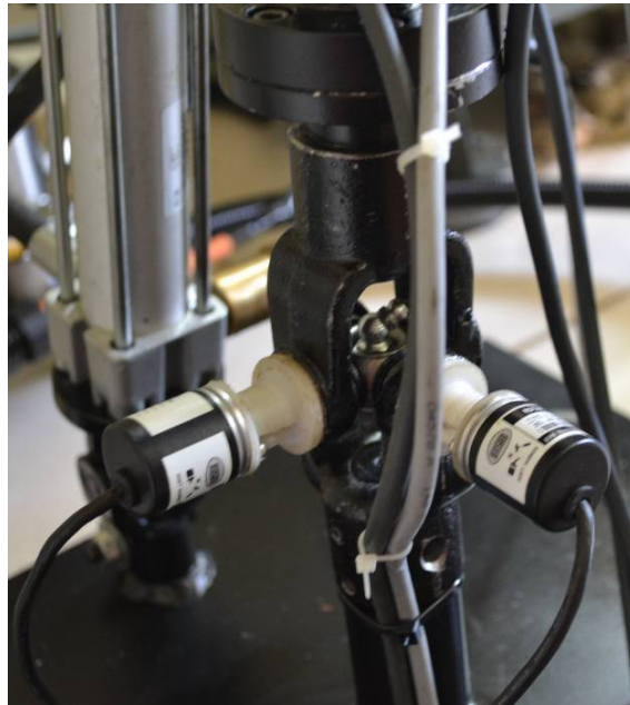
Figure 3.2: Universal joint with encoders.
