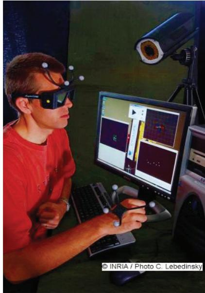
Figura 2.1: *CYCLOPE*<sup>7</sup> optical tracker.
