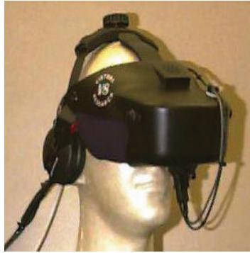
Figura 2.10: *HMD - Head-Mounted Display.*
