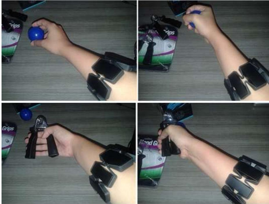
*Figure 19 Fist gesture holding a rubber ball and a hand grip*
