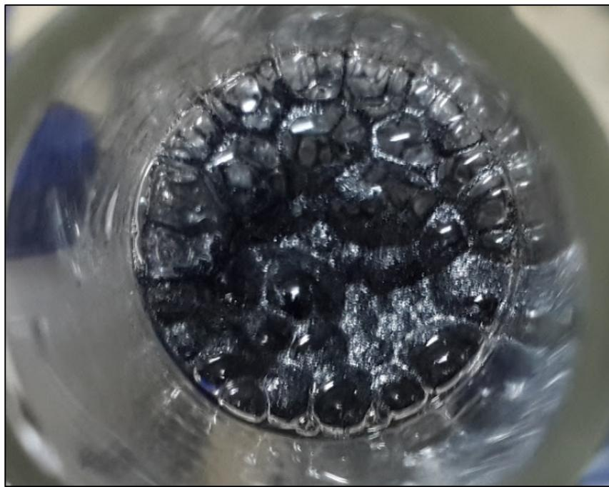
Photo A-5: Biosurfactant froth with hematite particles (+75 -150  $\mu\text{m}$ ),  $\text{NaCl}$   $10^{-3} \text{ M}$ , and concentration of 125 ppm and pH 3.
