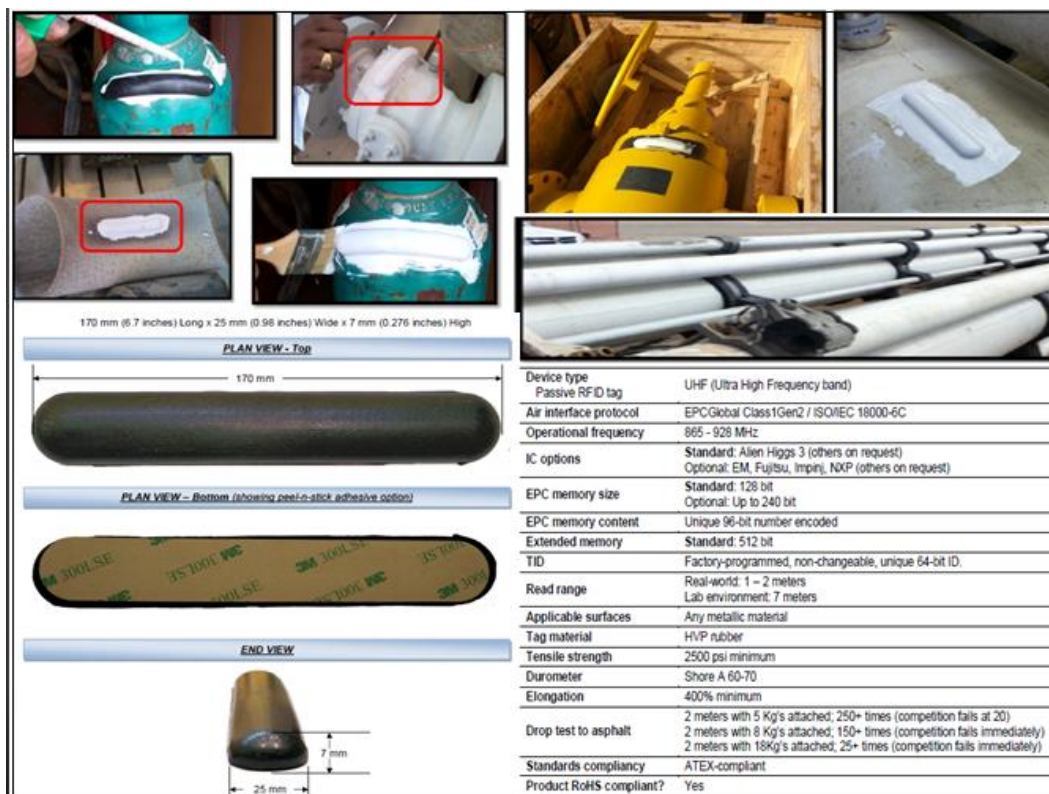
Figura 44: Exemplos de tag on metal adhesive-backed large pipe / cylinder
