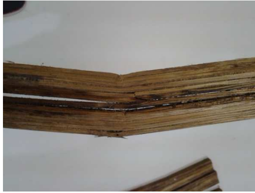
Figure 52 fracture on specimen 17 by brash tension and inner compression.
