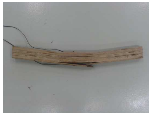
Figure 51 Fracture on beam specimen 3 by splintering tension and horizontal shear.
