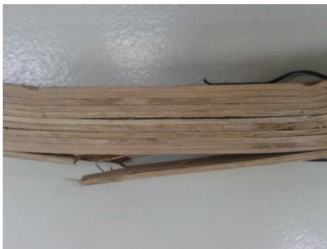
Figure 51 Fracture on beam specimen 3 by splintering tension and horizontal shear.
