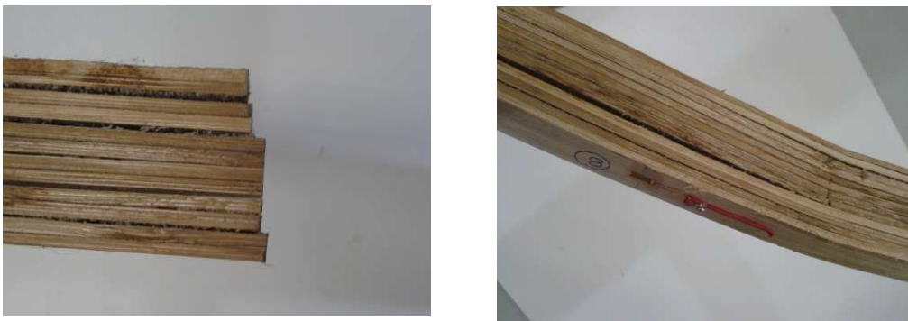
Figure 53 Fracture on specimen 8 by simple tension and inner compression.
