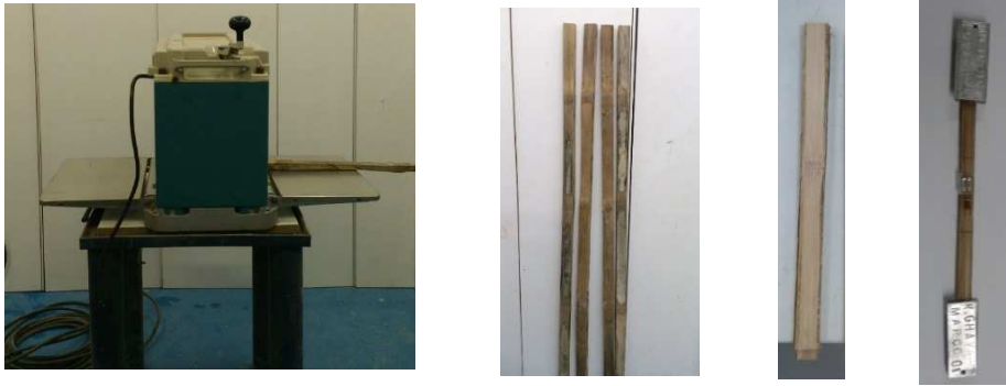
Figure 22 Thicknesser process to reduce and flatten strips into test specimens.
