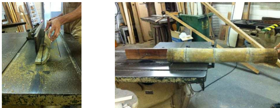
Figure 21 Splitting longitudinally bamboo culm to obtain strips.
