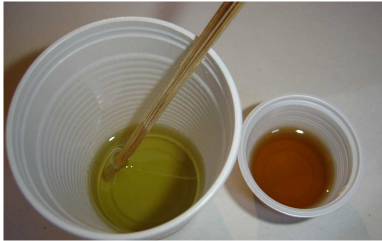
Figure 30 Image of mamona components Polyol and Pre-polymer and its respective proportions.
