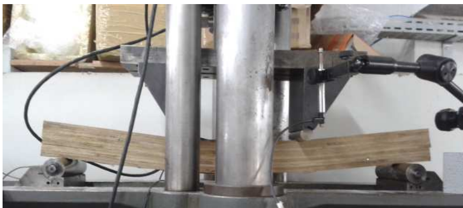
Figure 29 Picture of a 4 points bending test arrangement showing the load and supporting conditions.
