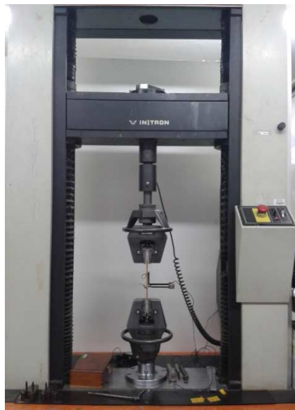
Figure 18 Hydraulic machine testing Instron 5500R.
