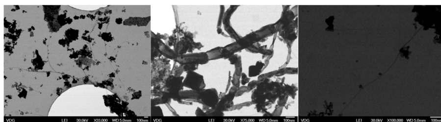
Figure 30: STEM images of Experiment Run 4 sample. On the left panel, there is a typical image of the sample. On the center panel, one can see some defective MWNTs, which will impact Raman spectra. On the right panel, there is a possibly SWNT bundle.
